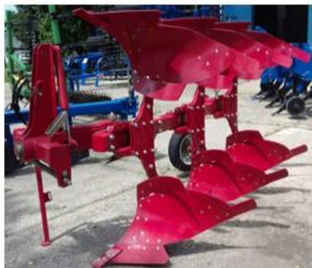
Fig. 6. Plug reversibil PR 3.
