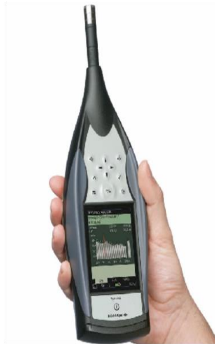
Figure 2. Sound Level Meter Bruel&Kjaer 2250 Light.
