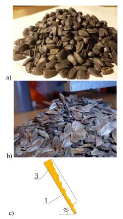
Figure 1. Aspects of the process of measuring the angles  $\alpha$  and  $\alpha_1$ : a), b) cones of seeds (*Silphium perfoliatum*, *Helianthus annuus*), c) the inclined surface with seeds
