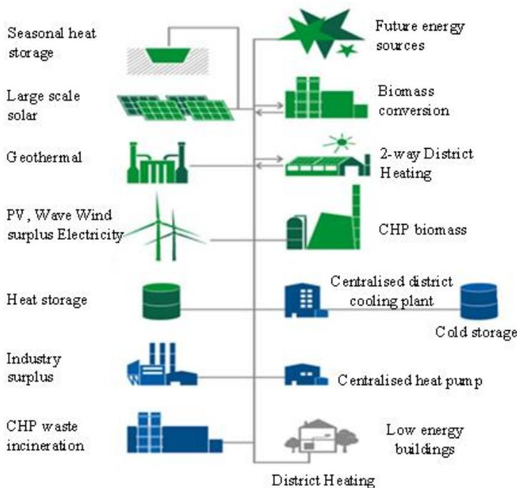
**Figure 1.** The constituent elements of a modern DHS, 4th generation [2]
