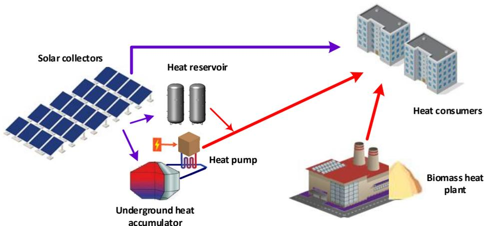
**Figure 5.** The component elements of a modern heating system
