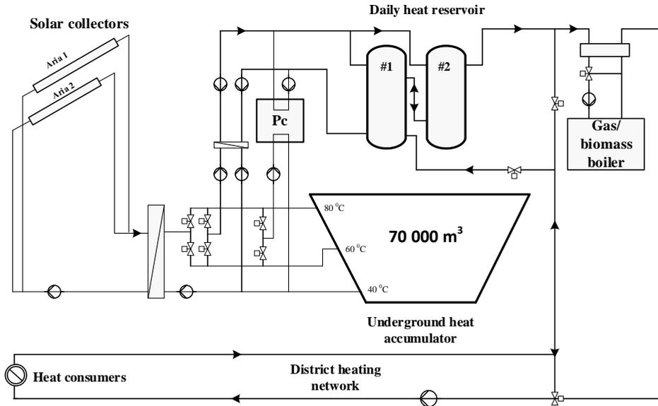
**Figure 10.** Integration scheme of solar collectors and biomass boilers in a heating system
