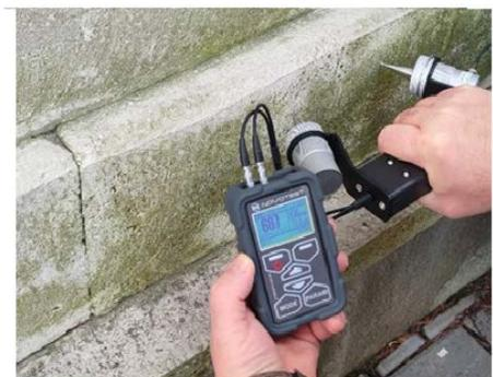
**Figure 2.** Ultrasonic pulse velocity tester.
