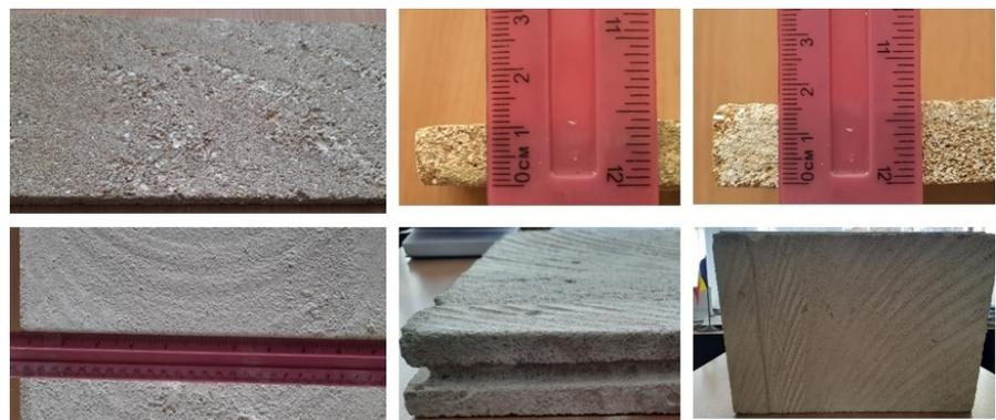
Figure 4. Limestone cladding for facade rehabilitation.
